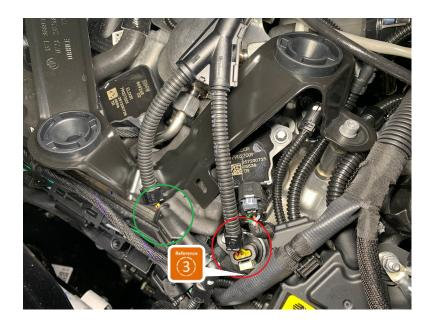
Localise the 3-pin camshaft sensor. Connect the adapter cable in between camshaft sensor and sensor plug.
