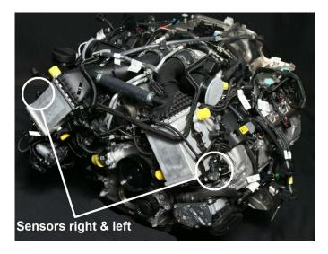
Localise the boost pressure sensor at the intercoolers (left and right).
