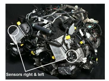
Localise the boost pressure sensor at the intercoolers (left and right).
