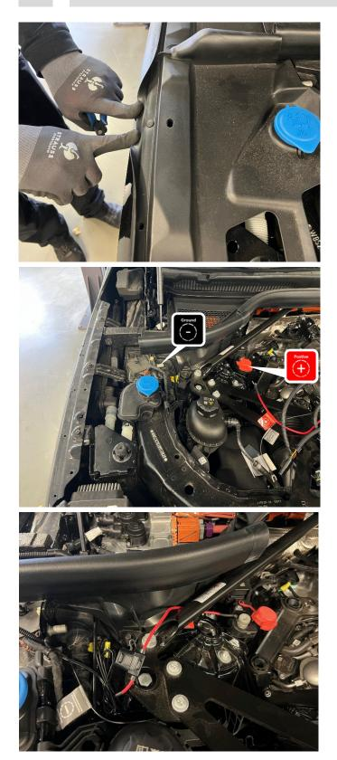
Open all plastic clips to remove the cover on the left side.
