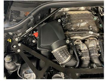
Disconnect the boost pressure sensor connector by unlocking the locking lever from the boost pressure sensor. Connect the adapter cable in between these connection.
